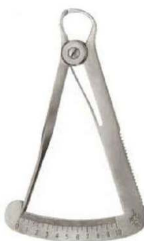
RW-1452 Fig. 2 Iwanson spring caliper For wax.
